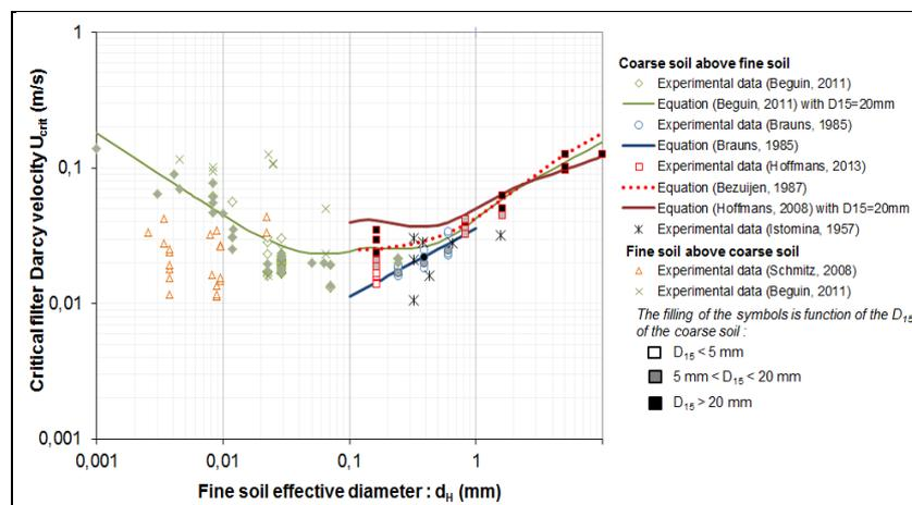
Figure 1. Darcy velocity in coarse soils to cause contact erosion of fine soils at the interface (Figure 5.2 in ICOLD, 2015, courtesy of Dr Remi Beguin (Beguin, 2011))
