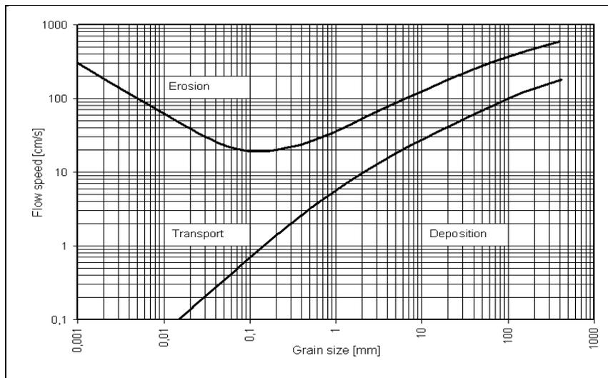
Figure 3. The Hjulström (1939) version of the Shields diagram
