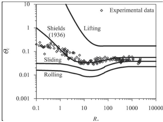
Figure 2. Threshold Shields function  $\Theta_c$  versus shear Reynolds number  $R^*$  in rolling, sliding and lifting modes (from Figure 6, Dey and Ali, 2016)
