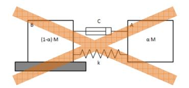
This simple model is no longer valid: it should model the total momentum at the foundation, not the shear force
